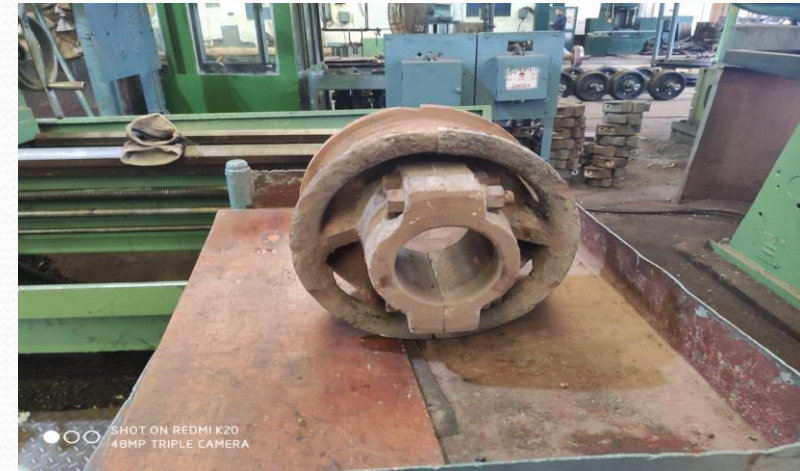
Existing Cast Iron Pulley (wt - 52 kg.)
