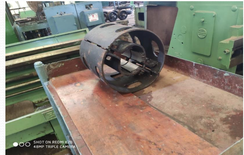
Newly developed fabricated Pulley (wt - 28.5 kg.)
